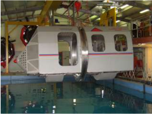
The EDM manufactured HUET at the pool facility of the Fleetwood Offshore Survival Centre in both the upright and inverted submerged positions.
