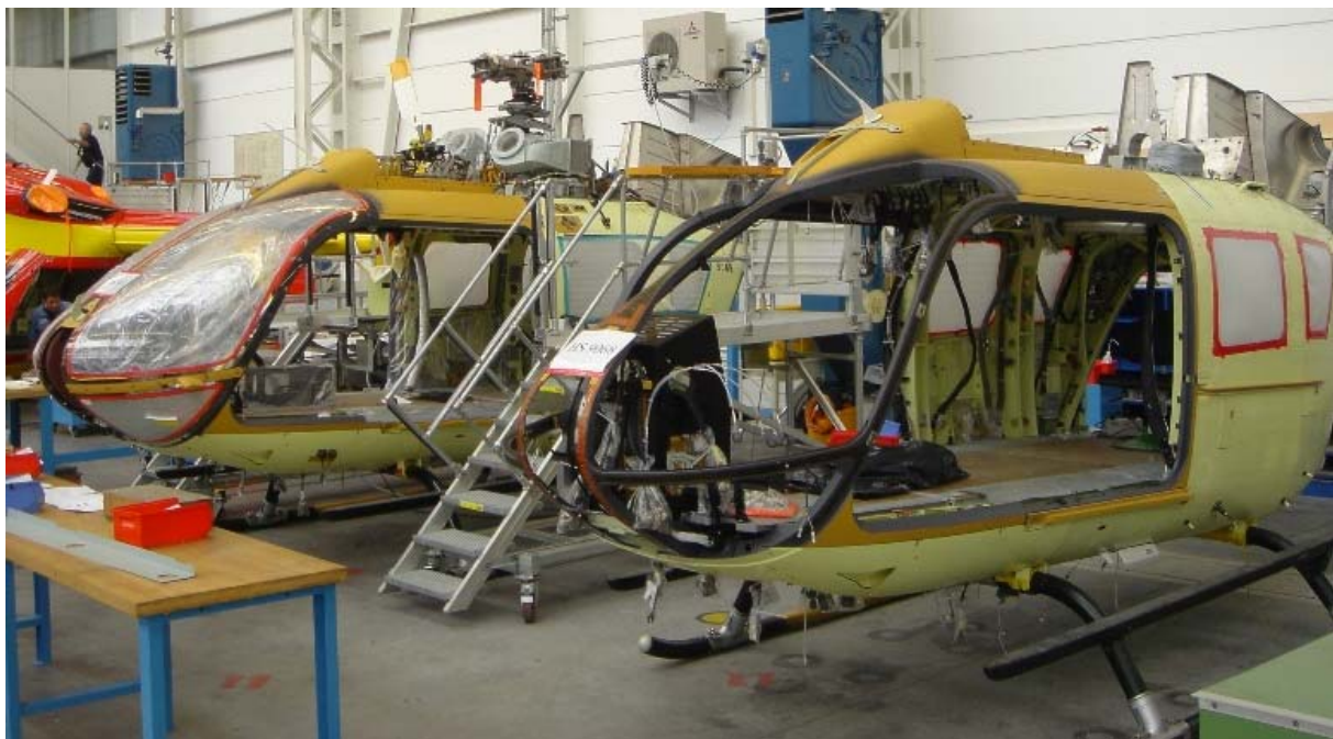
BK117C2/EC145 c/n 9065 and 9068 on the Donauworth production line. Images via MPS
