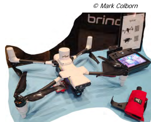
The AVSS parachute recovery system is the white canister on top of the drone © MC
