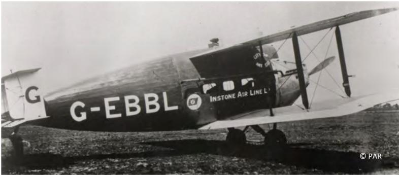
The 360hp Rolls Royce Eagle engine was insufficient power for the bulk of the Vulcan, leaving it under-powered and incapable of carrying its designed load of passengers to its intended destination, France. Less than a dozen Vulcan's were built, most of the purchasers sending them back to the manufacturer after a brief acquaintance. The blue and silver Vulcan the police used, G-EBBL, had originally served as the prototype prior to service with Instone Airline Ltd. It first flew in
