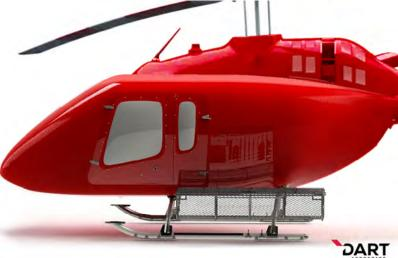
Through the Airbus EC135 retrofit, all equipment is contained in a rugged roll-on-/roll-off rack, which can be installed in the helicopters within 5 minutes, with seat-rail quick-locks attached to the airframe, and easily connected to the helicopter's standard power outlet and the video-cameras to 3G-SDI video outlets.
