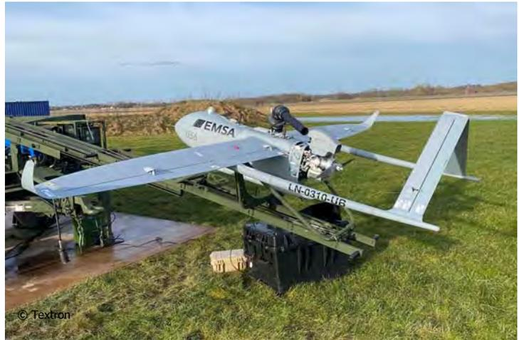
EMSA is providing this service through its contractor Nordic Unmanned, deploying a Textron Aerosonde which uses a catapult for take-off and a recovery net for landing. The Textron Aerosonde unmanned fixed-wing aircraft can stay in the air for 10 hours and can fly up to 140 km within radio range and further depending on the ground relay stations. The aircraft is equipped with a gimbal with optical and infrared sensors, AIS receiver and IMSAR radar.
